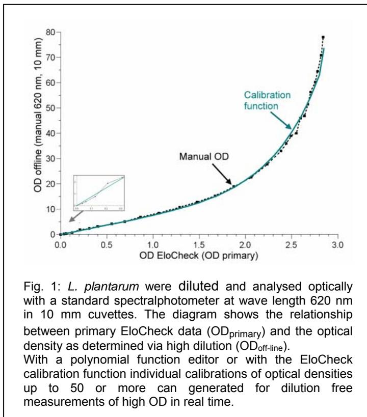
*Correct measurement of OD without any dilution.*
