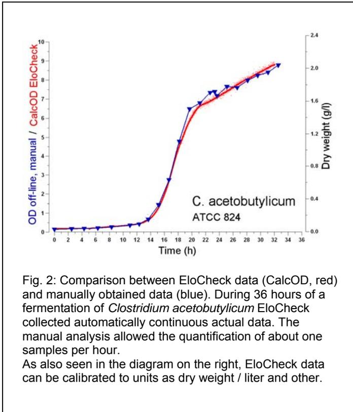
'OD<sub>off-line</sub>' is often called 'off-line laborious optical density'. Here it represents the optical density as quantified via high diluted samples. In such highly diluted samples scattering errors are negligible and the resulting OD<sub>off-line</sub> is proportional to the particle concentration.
