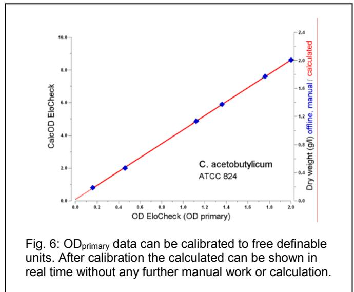
Fig. 6: OD<sub>primary</sub> data can be calibrated to free definable units. After calibration the calculated can be shown in real time without any further manual work or calculation.
