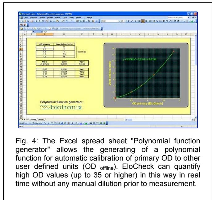
Fig. 4: The Excel spread sheet "Polynomial function generator" allows the generating of a polynomial function for automatic calibration of primary OD to other user defined units ( $OD_{\text{offline}}$ ). EloCheck can quantify high OD values (up to 35 or higher) in this way in real time without any manual dilution prior to measurement.
